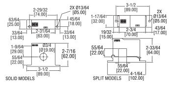
The Series CCT40/50 Current Transformers are a low cost alternative for measuring power and monitoring the operation of fans, pumps, and other equipment. Series CCT60/70 True RMS Current Transformers provide true RMS outputs on distorted AC waveforms. Split core models can be installed without disconnecting cables. Each model offers three jumper selectable ranges and a choice of three different outputs.
